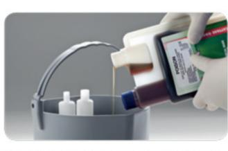
Unscrew and remove the red cap. Pour the solution from the dispensing cup into the full Pulse Cleaner. Take care to not allow more solution from the main bottle flow into the dispensing cup.
